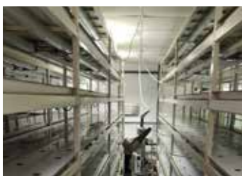
Bioquell RBDS deployed during crop changeover
